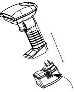
*Note:* Recharge Time: 6 hours at any voltage at 20°C (68°F.)
